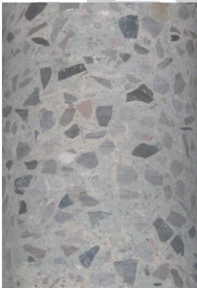
A concrete core from a Logix wall
